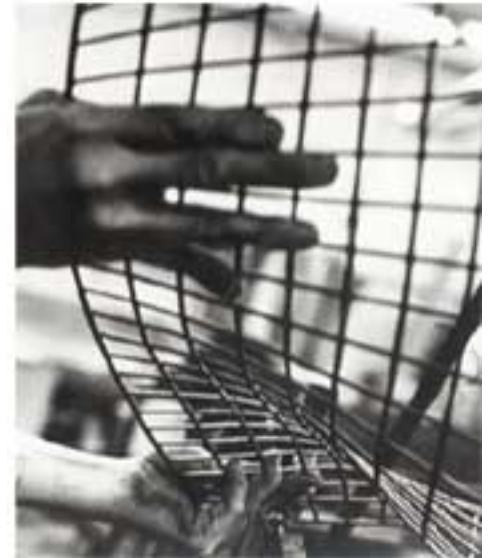
Bertoia chair shell frames are still made by hand
